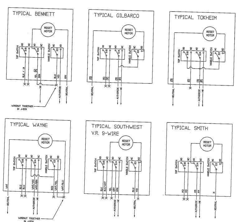
AUTHORIZE - provides the 115 VAC HOT to the reset motor; it is also used to detect the call signal.
