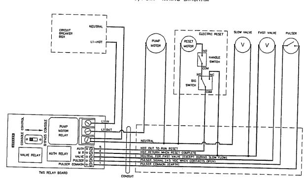
TYPICAL TMS/PUMP WIRING DIAGRAM
