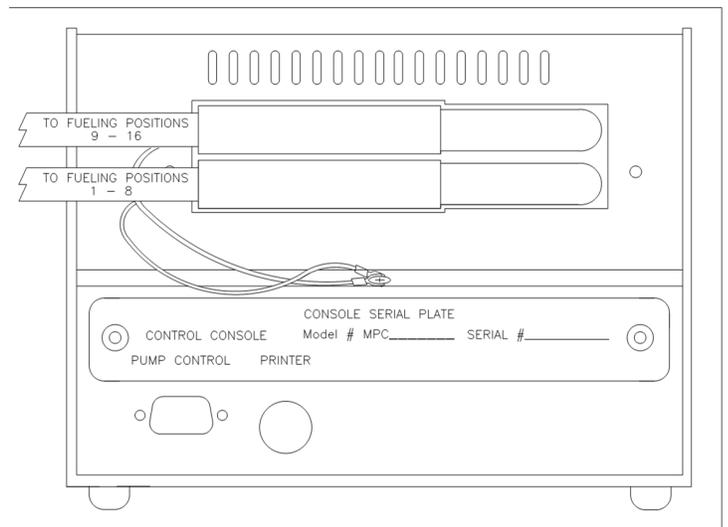
Figure 5. Hybrid console with two mechanical IF boards
